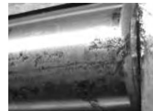
Fig. 190. Pitting on roller.
