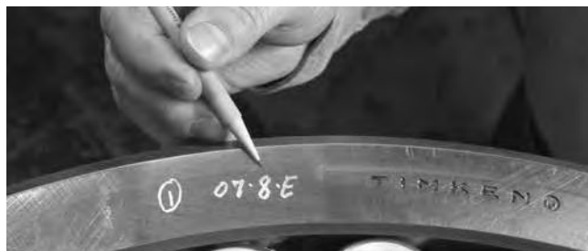
Fig. 266. Example of E cup marking.
