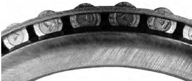
Fig. 183. Roller end and rib discoloration.
