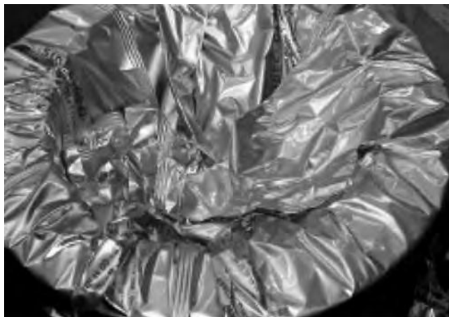
Fig. 194. Vacuumed and hot-sealed aluminum foil bags for large bearings.
