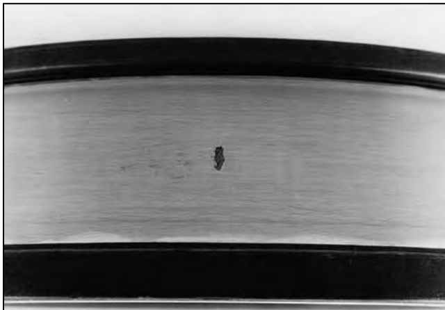
Fig. 169. Inclusion origin spalling.
