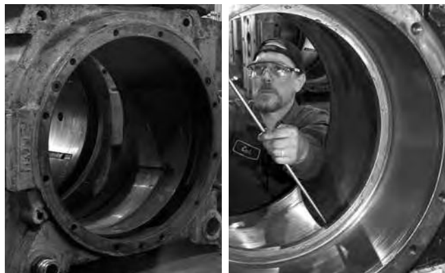
Fig. 278. Chock maintenance before and after photos.
