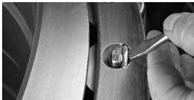
Fig. 231. Removing locking wire from an inspection pin.
