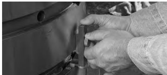
Fig. 268. Measuring B or D gap.
