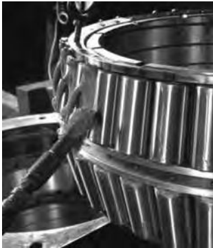
Fig. 245. Lubricating a tapered roller bearing with grease.
