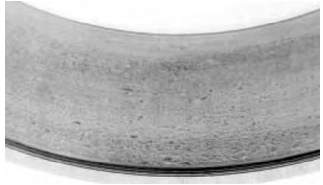
Fig. 160. Bearing damage due to abrasive particles.
