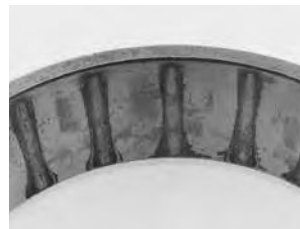
Fig. 189. Staining without pitting.
