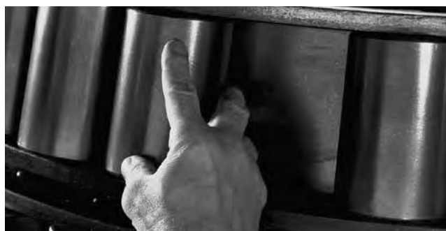
Fig. 233. Inspecting cone race.
