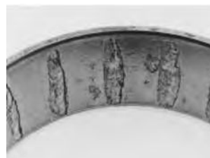
Fig. 191. Deep etching on an outer ring race.
