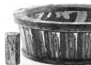
Fig. 192. Damage caused by poor storage conditions.
