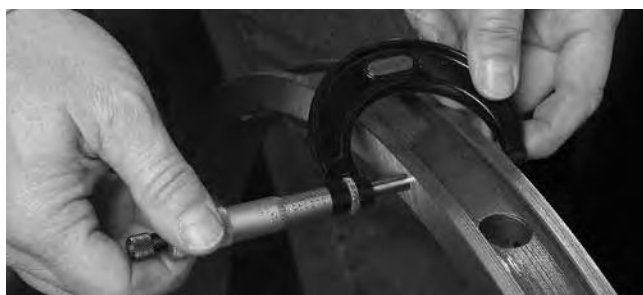
Fig. 269. Measuring spacer width.
