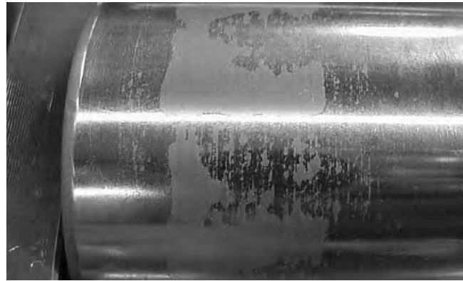
Fig. 184. Roller peeling damage.
