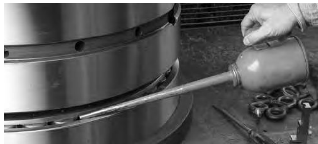
Fig. 267. Applying light oil to rollers and race.
