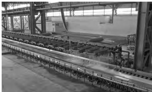
Fig. 110. Hot-strip mill roller tables.
