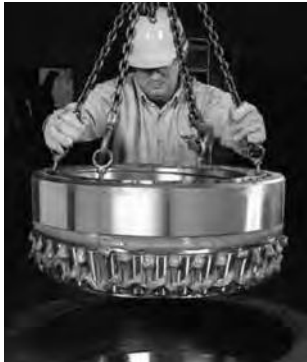
Fig. 246. Installing a greased roller component in the chock.
