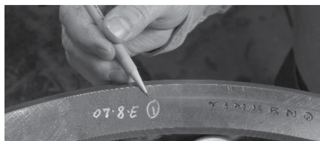
Fig. 226. Example of quadrant marking.
