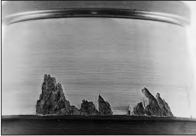
Fig. 171. Geometric stress concentration spalling.
