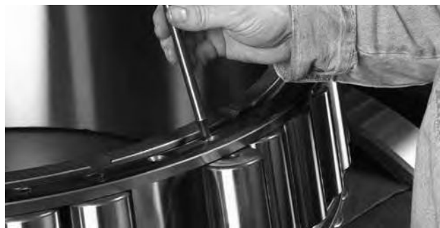
Fig. 232. Removing the threaded pin.
