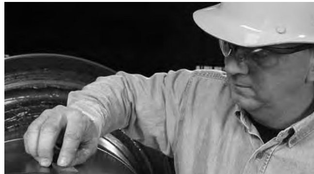
Fig. 240. Restoring minor roll neck damage.
