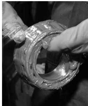
Fig. 51. Grease can easily be packed by hand.
