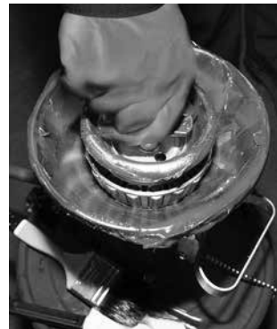
Fig. 52. Mechanical grease packer.
