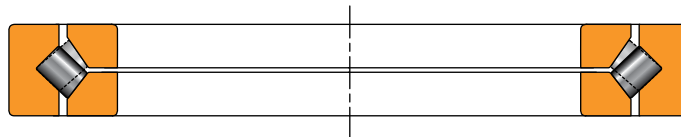
Fig. 24. Type TXR crossed roller bearings.
