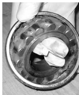
Fig. 21. Grease can easily be packed by hand.
