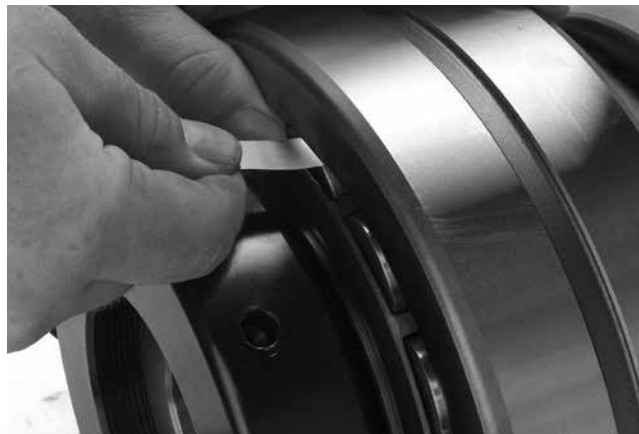
Fig. 7. Measure RIC before installation.
