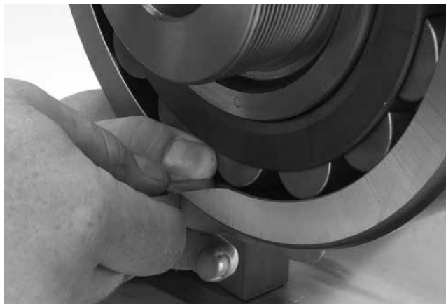
Fig. 4. During mounting, the RIC should be checked at the unloaded roller.
