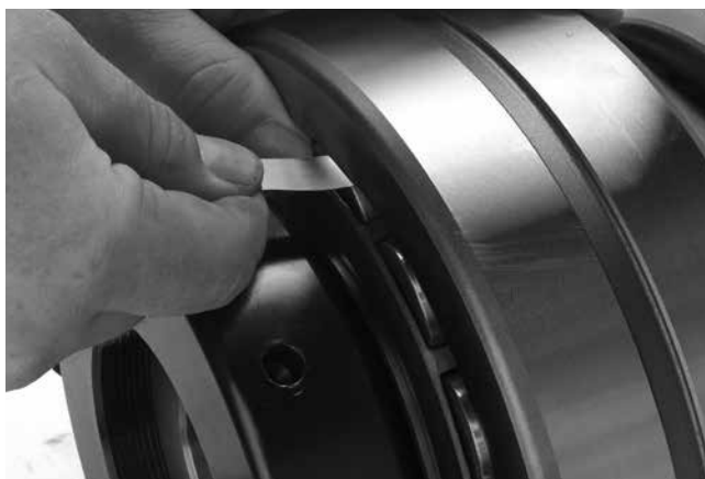
Fig. 3. Measure RIC before installation.
