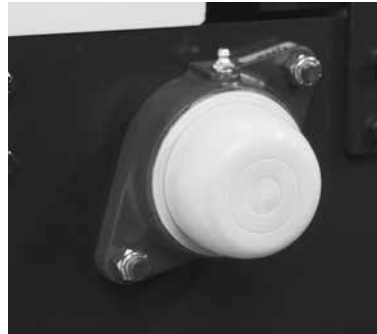
Fig. 29. Safety end caps protect against rotating stub shafts.
