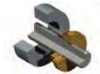
Figure 16: Flanged Seal Flush with Housing Face
