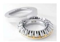
Timken designed type TSR thrust spherical roller bearings to achieve a high thrust capacity with low friction and continuous roller alignment. This bearing type is ideal for operating conditions that experience heavy loads, difficulty in establishing or maintaining housing alignment, or shaft deflection.
