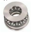
The TPS type thrust cylindrical bearing is similar to type TP, except the bottom washer is comprised of two races, with the contacting faces spherically ground. The TPS bearing is self-adjusting to initial misalignment. It is not suggested for applications where alignment may be continuously changing (dynamic misalignment).
